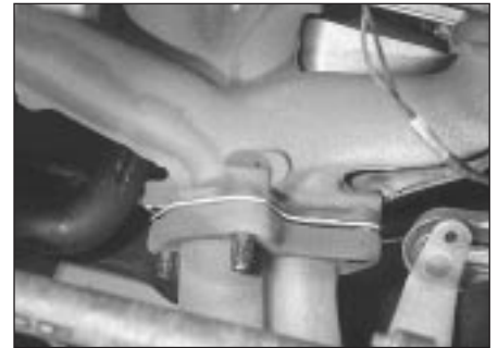
25.3b Exhaust manifold-to-downpipe connection - BX 16
