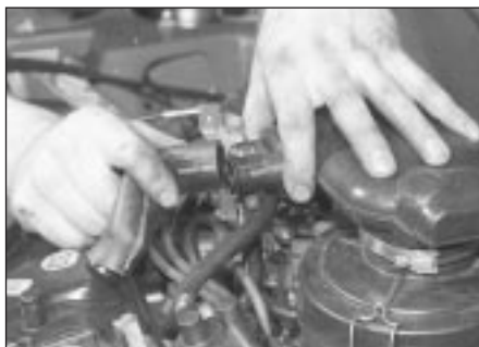
3.3a Disconnecting crankcase vent hose from air cleaner
