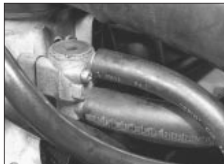
14.9 Solex 32-34 - ventilation hose connections
