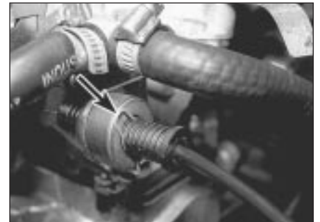
23.2 Solex carburettor - accelerator cable location bracket. Adjustment/securing clip of outer cable is indicated
