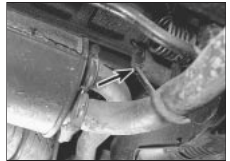
26.3 Exhaust system flexible hanger (arrowed)
