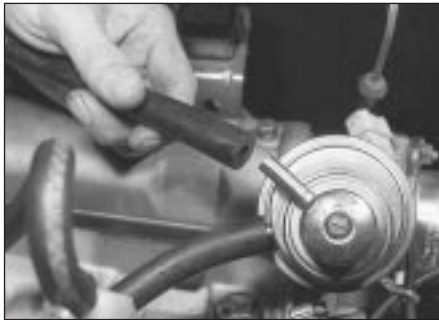
7.1 Fuel supply hose removal from fuel pump
