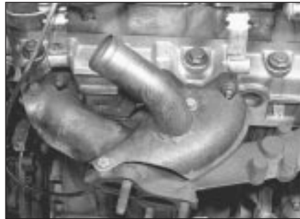
25.3a Exhaust manifold with air filter hot air collector cowling fitted - BX 16
