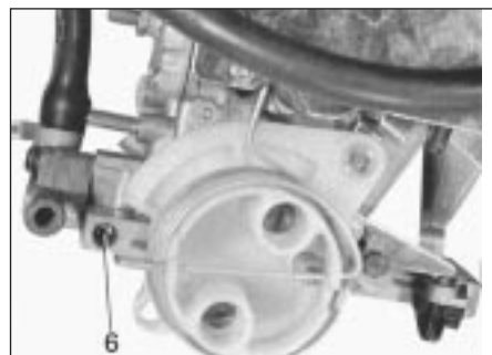
13.5a Solex 32-34 - mixture adjustment screw location (6)
