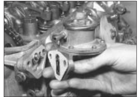
7.3b Fuel pump removal - BX 14
