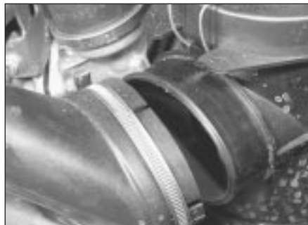
3.2a Air intake disconnected from air cleaner casing
