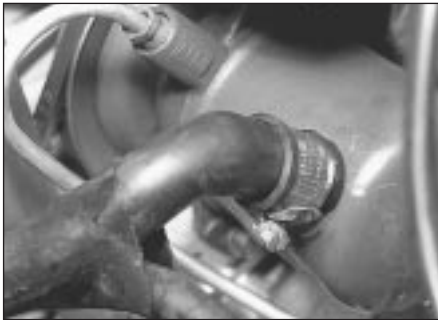
5.3 HP pump showing the supply and output pipe connections
