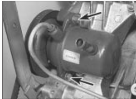
5.4 Detach the output pipe. Pump retaining bolts arrowed
