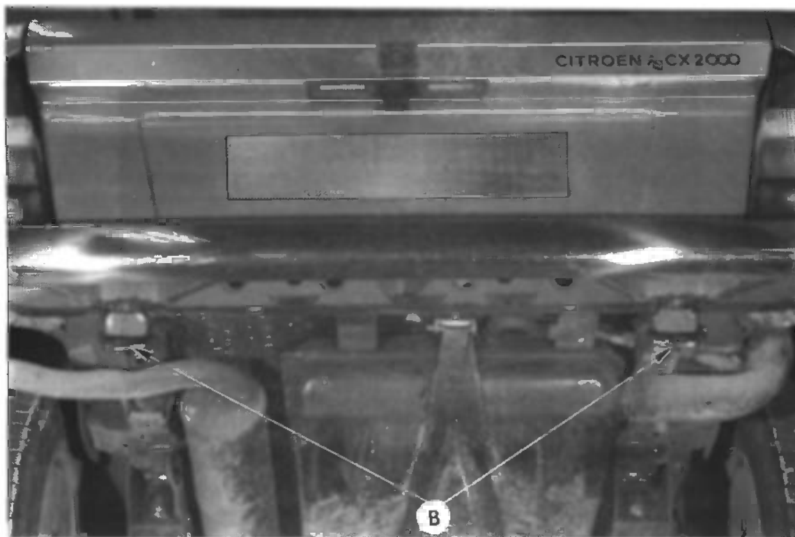
B - Towing eyes on the rear bodyshell sidemembers
