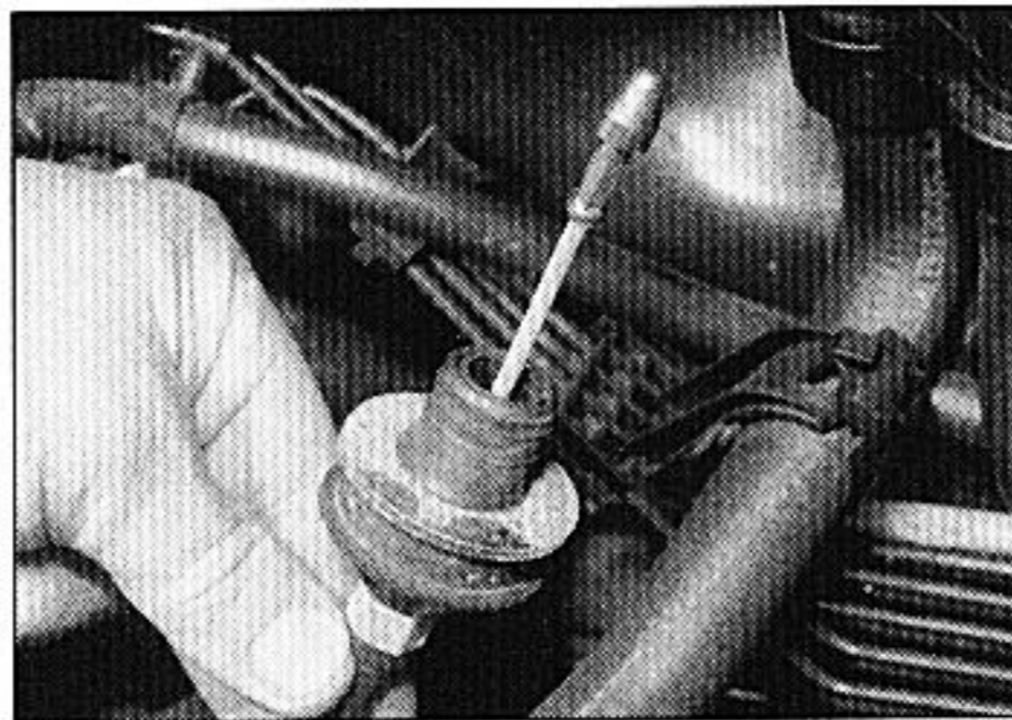
3.8a Inserting the clutch cable through the bulkhead. Note the inner cable end fitting which locates in the plastic clip
