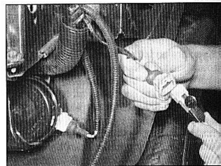
8.8 Disconnecting the foglight wiring connector
