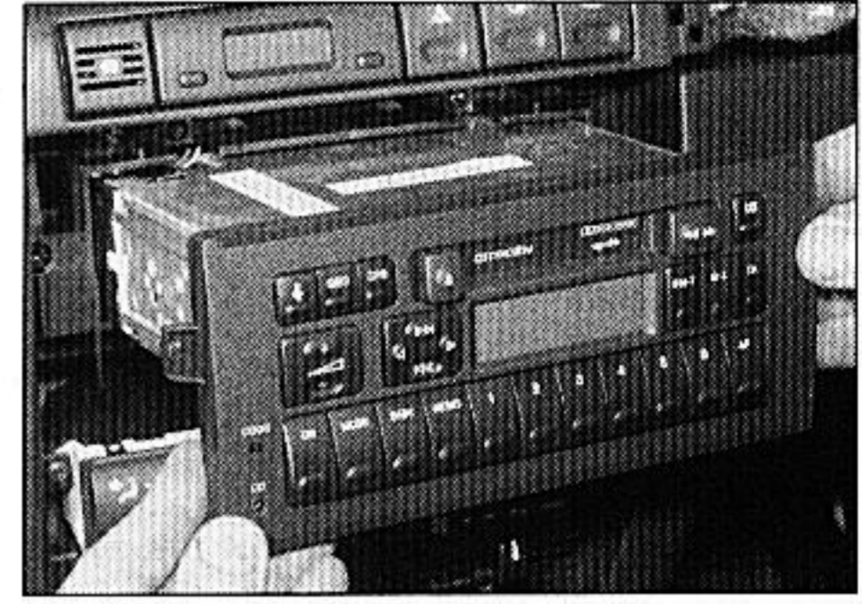
20.4b . . . and withdraw the radio/cassette player
