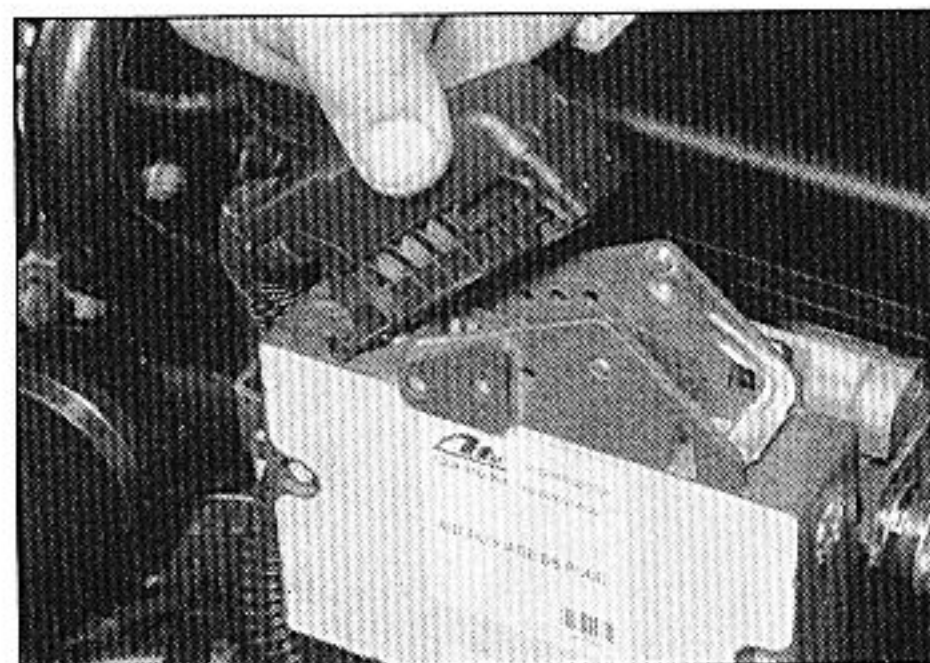
16.28 Disconnect the ABS control unit wiring plug
