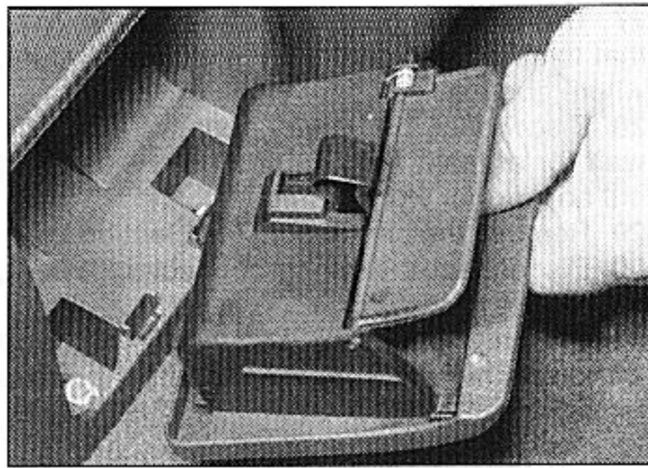
26.6 Unclip the ashtray from the centre console
