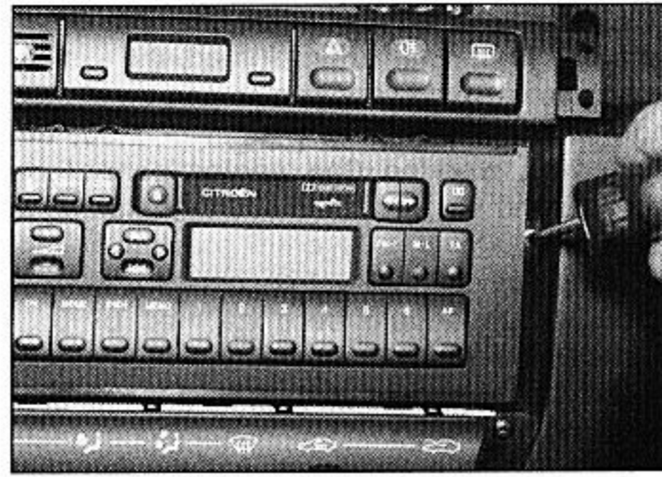
20.4a Remove the two securing screws (one each side) . . .
