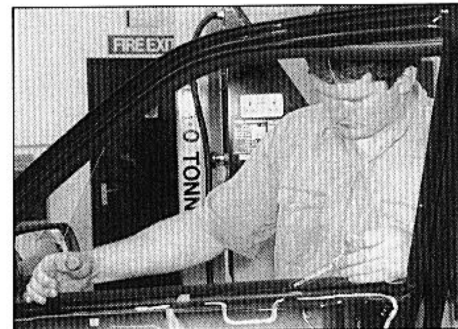
14.6 Lifting out the front window glass
