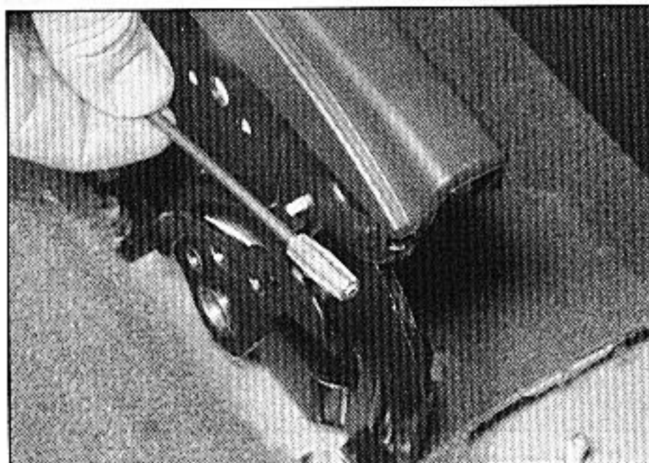
12.6 Unclip the handbrake cable from the lever
