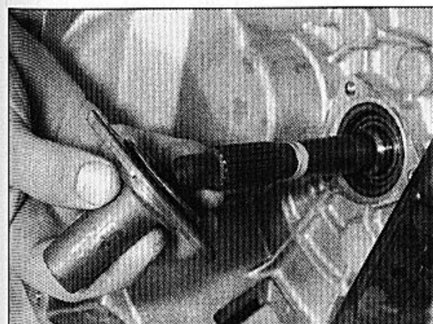
6.27b . . . and refit the guide sleeve over the input shaft
