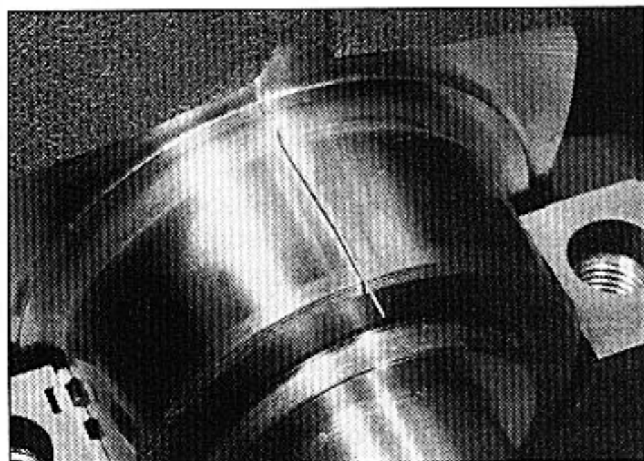
19.17 Plastigauge in place on a crankshaft main bearing journal
