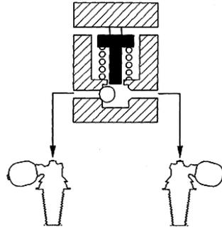
In the picture above, a situation is shown where the vehicle is making a left turn, and tends to roll to the right. This compresses the right strut and expands the left strut, causing a cross flow of fluid, from the compressed strut to the expanded one. This moves the ball in the valve towards outlet to the left strut, closing off further cross-flow. The remaining damping is left to the spheres on the strut.
