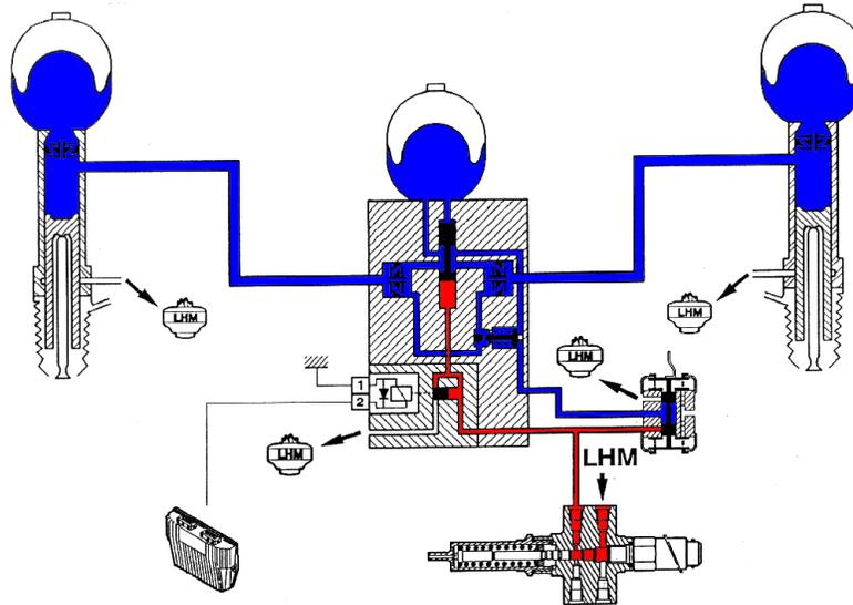
The picture above depicts the soft setting of the control block. The blue areas are LHM fluid under suspension pressure, the red area is the suspension hydraulics feed, under the system feed pressure (equal to the main accumulator pressure under normal operation).
